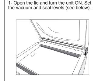
2- Lay the pouches on the shims and align their opening along the sealing cushion.
